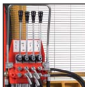
Distributore 4 leve Distributor with 4 levers
