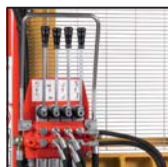
Distributore 4 leve Distributor with 4 levers
