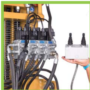
Distributore elettro-idraulico Electro-hydraulic distributor
